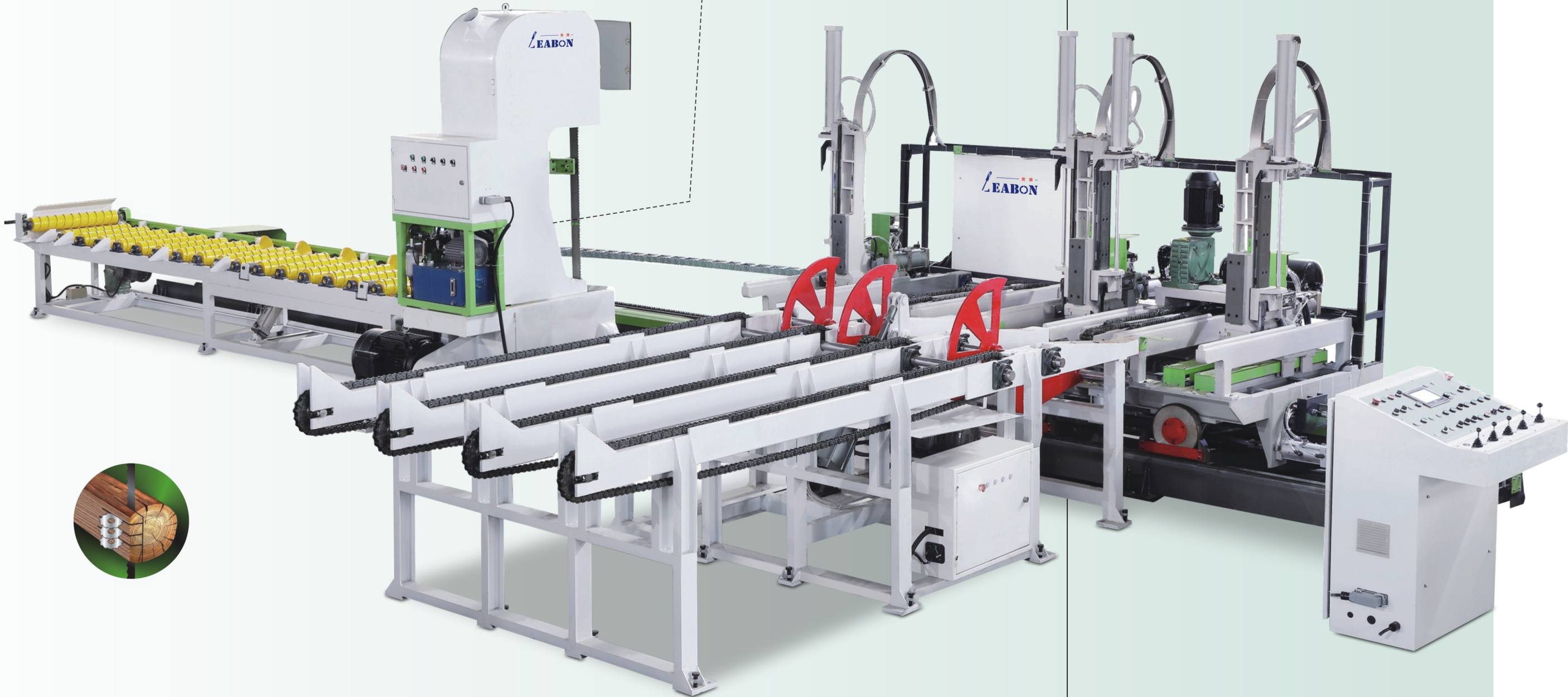
It can be equipped with multiple saws, and the horizontal and vertical surfaces can be sawed at the same time
