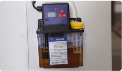
Automatic Oiling Lubrication System, Ensure The Guide Rail Lubrication And Wear Resistance
