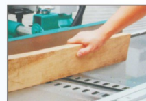
Manual Planing is Possible and is Suitable for Single-piece Processing
