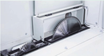
Large And Small Saws Start Independently And Lift Vertically
