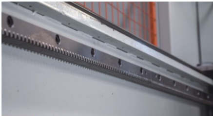
The Saw Truck Transmission Uses Rack And Pinion And Servo Motor
