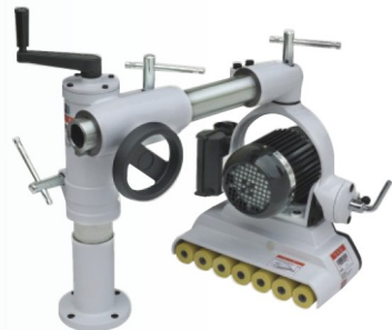
Ring Type Small 7 Wheels Feeder (For Short Material)
