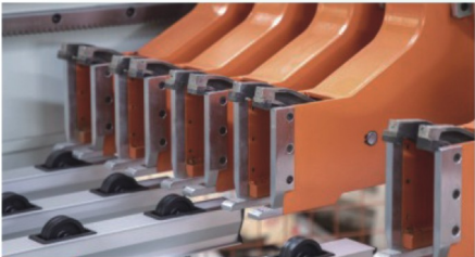
The Robot Automatically Feeds The Material, And The Double Clamps Stabilize The Material Grabbing
