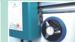
Angle to be Adjusted by Hand Wheel
